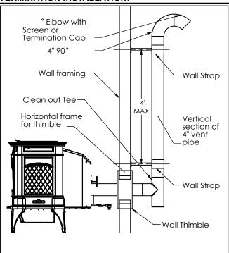
THROUGH CONCRETE WALL WITH VERTICAL RISE INSTALLATIONS:
