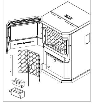
Figure 12: Firebox Components Removal.
