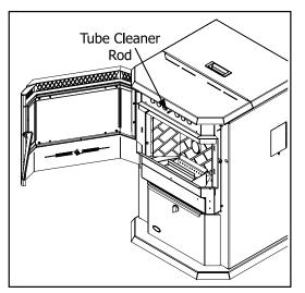
Figure 11: Heat Exchanger Tube Cleaner.
